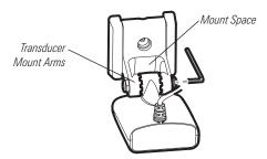
2. Push the Transducer Insert up through the mount space until it is fully inserted. If the space is not easily accessible, lift up the transducer.
