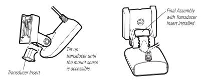
3. Once the Transducer Insert is fully installed, reposition the transducer and tighten the mount arms. Adjust the transducer for on-the-water operation as needed (see your transducer installation guide for details).
