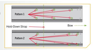
**NOTICE:** If Pattern 2 is used, the right side plate must be removed using a #2 Phillips Screwdriver to access the mounting holes in the base of the Mount.
