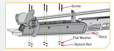
NOTICE: To prevent seizing of the stainless steel hardware, do not use high speed installation tools. Wetting the screws or applying an anti-seize may help prevent seizing. If possible, secure all sets of mounting bolts, nuts and washers.
