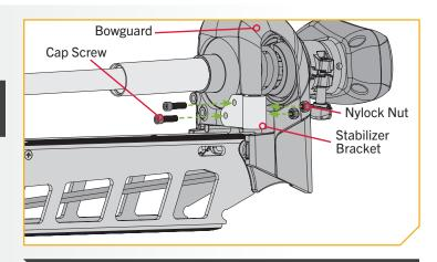
**NOTICE:** The two Lock Washers (Item #32) are not used when installing on the Fortrex.
