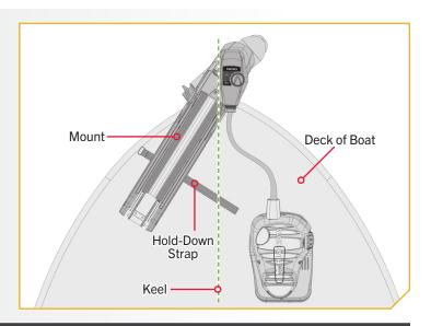
**NOTICE:** Check that the Motor can properly stow and deploy at the intended mounting location. The Mount should latch closed when deployed. A proper deployment requires engaging the Pull Grip and Rope when the Motor is stowed to unlatch the Mount. If the latch on the Mount does not engage when deployed, it could indicate that the Mount is not flat on the Boat Deck. Use rubber washers to level the Mount on the Boat Deck if the Mount is not latching when deployed.
