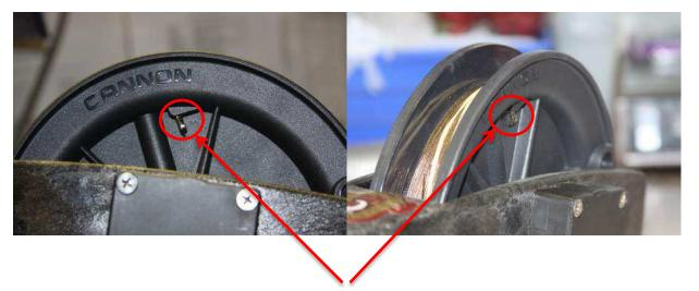
The pictures above show the hole location on the spool and where the sleeve will be crimped onto the cable.
