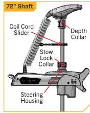
unlocked to allow the Shaft to move freely when stowing and deploying. After stowing the motor, the Stow Lock Collar is locked to ensure a secure stow. The Stow Lock Collar can also be locked to hold the motor at the proper depth when deployed in shallow water.
