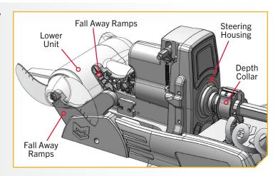
**NOTICE:** To secure the motor in place and prevent accidental deployment when stowed, slide the Depth Collar down against the top of the Steering Housing and close the Cam Lever to lock the Depth Collar.
