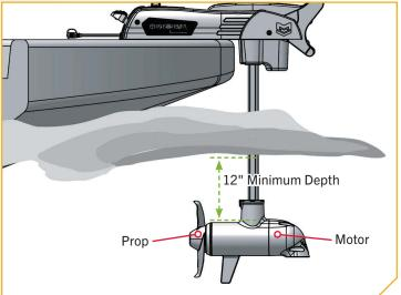
**NOTICE:** Ensure that the top of the lower unit is submerged at least 12" below the surface of the water to avoid churning or agitation of surface water.
