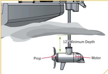
**NOTICE:** Ensure that the top of the lower unit is submerged at least 12" below the surface of the water to avoid churning or agitation of surface water.
