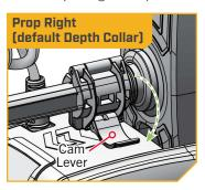
If the Stow Orientation is changed to Prop Right, the Depth Collar must be rotated on the shaft to improve accessibility. The Depth Collar is positioned correctly on the Shaft when the Cam Lever opens upward when the motor is stowed.
