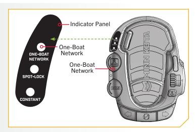
NOTICE: While the Raptor/Talon is deploying, the action can be paused by pressing the One-Boat Network button on the Foot Pedal.
