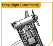
A Prop Right orientation turns the lower unit and shaft when stowed, causing the Depth Collar to open downward. This reduces its range of motion and creates an obstruction when placing the Depth Collar for a secure stow.
