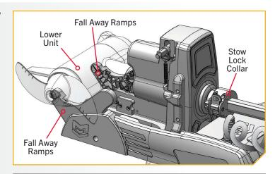
**NOTICE:** To secure the motor in place and prevent accidental deployment when stowed, lock the Stow Lock Collar . Be sure to press the Lock Arm so that it is fully seated against the Stow Lock Collar.
