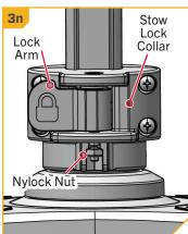
**NOTICE:** If the Stow Lock Collar is too tight, the Shaft will not move freely even when the Stow Lock Collar is unlocked. If the Stow Lock Collar is too loose, it will not securely hold the Shaft when locked.
