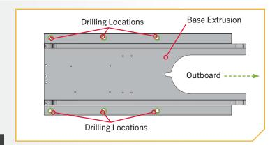
**NOTICE:** The mounting surface for the Terrova QUEST must be flat. Rubber Washers can be used to shim the Base Extrusion flat before hardware is tightened.
