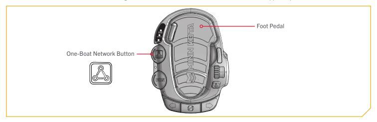
The One-Boat Network A button on the Foot Pedal can be customized to control the following functions:
