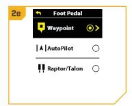
NOTICE: The radio button next to the desired function will be selected when the Steer Right 💆 button is used to customize the function. AutoPilot is the default selection for Terrova QUEST trolling motors. The function options listed are based on the trolling motor and other devices in the Advanced GPS Navigation network.
