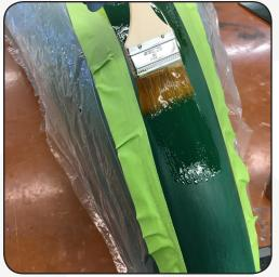
5. With a disposable paint brush, apply mixed resin to the sanded area, covering it completely with resin.
