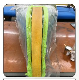
7. Apply as much resin as necessary to completely wet through the felt. Use the brush to work any trapped air out from under the felt.
