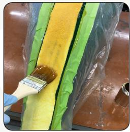
6. Lay the Kevlar Felt(A) carefully in place. Pat it firmly with your gloves hand or paintbrush to begin wetting the felt with the resin underneath.
