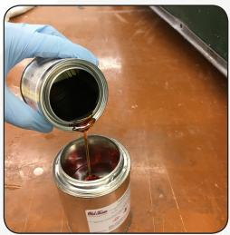
4. WEARING GLOVES, mix the resin by pouring all of Can-B Hardener(C) into Can-A Resin(B). Stir thoroughly with a stirring stick. Make sure to scrape the inner sides of the can to achieve uniform mix.
