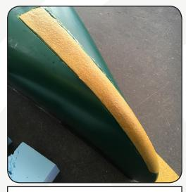
10. Allow the skid plate to cure for 24 hours. If desired, the resin may be lightly sanded after curing for a smooth finish.
