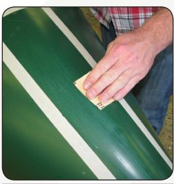
2. Remove the skidplate(A) and sand the masked area with the 40 grit sand paper(D) provided. Look carefully at the surface for any shiny areas showing missed spots. Sand those areas again. Wipe free of debris with a clean dry cloth.
