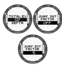
The SIF can be selected from 5 to 20 or disabled with the OFF setting by pressing the +/UP or -/DOWN buttons and then the SEL/ESC button to save.
