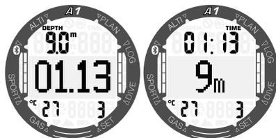
During the Apnea dive these two screens show the current dive depth and duration and they can be scrolled through by pressing the +/UP or -/DOWN buttons.
