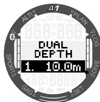
Both depth alarms can be set from 5 to 100 meters (20 to 330 feet) in 1m/5ft increments by pressing the +/UP or -/DOWN buttons. By pressing the SEL/ESC button the first value is confirmed and the second depth can be adjusted.
