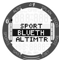
At this point the A1 is ready for Bluetooth communication. Bluetooth is active only when this screen is displayed.
