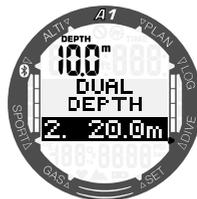
The value of the second alarm can be set the same way as that of the first alarm. In the upper left section of the screen the depth of the first alarm is displayed.
