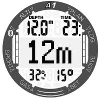
Current depth is shown in feet or full meters without a comma. This is the larger duplicate of the top row depth.
