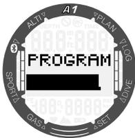
Once the new software has been programmed, the A1 will complete a few internal checks and perform a reboot.
