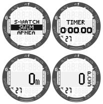
When the swim mode is activated, the duration of your swim will be shown on the second screen. The distance will be displayed on the third screen and the last screen will show the number of swim strokes. The water temperature is shown in the bottom left of the display. Switch between displays by pressing the +/UP or -/DOWN buttons. A press of the SEL/ESC returns you to the **Sport** menu.
