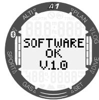
After a successful update the A1 will display the message "Software OK". This message can be cleared by a short press of the SEL/ESC button. After this your A1 is again ready for normal use.
