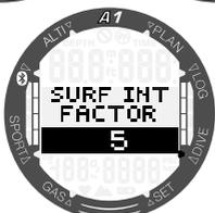
The SIF can be selected from 5 to 20 or disabled with the OFF setting by pressing the +/UP or -/DOWN buttons and then the SEL/ESC button to save.
