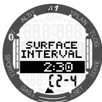
The prohibited altitude class is shown after the current elevation at the bottom line. For more information on altitude diving with the A1, see chapter 4.9 **Altitude diving**. In case the A1 is displaying the no-dive warning, the duration of the warning itself is displayed as a recommended surface interval for planning purposes (rounded up to the nearest 15-minute increment).
