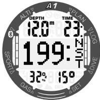
No-Stop Time, which is the time at current depth before decompression stops are required.
