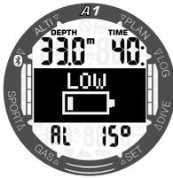
During the dive A1 will alert you if the battery level is getting critically low. This means you need to start the procedure to terminate the dive, as there is not enough energy in the battery to ensure the proper functions and the computer may fail. Some functions like backlight and audible alarms are no longer available.
