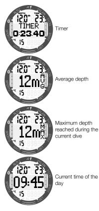
NOTE: In GAUGE and SCUBA mode when the timer is displayed, it can be stopped by a press-and-hold of the +/UP button. A repeated press-andhold of the +/UP button will restart the timer. When the timer is stopped, it can be reset to zero by pressing-andholding the -/DOWN button.
