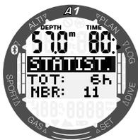
By pressing the SEL/ESC button you will enter the repository of the logs where you can scroll through your dives with the +/UP or -/DOWN buttons. The below display shows the following information: Dive number, dive mode, dive start time and date.
