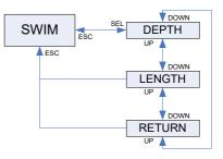
For the swim stroke counter you must set the cycle threshold—how much depth difference is counted as a stroke cycle, as well as the distance per cycle (stroke length)—to achieve the proper result.
