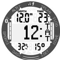
Total Ascent Time, which is the time to the surface with optimal ascent speed including the possible stops.
