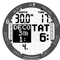
**NOTE:** When the A1 is in **GAUGE** or **APNEA** modes, the Planner is disabled and this is indicated by a display like the following:
