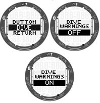
NOTE: Dive alarms are still active even if you switch the dive warnings off. Dive alarms are deactivated only when the buzzer is switched off as described in chapter 3.1.3.1 Buzzer.
