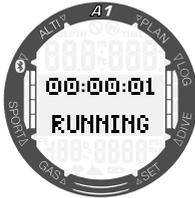
To pause the time on the stopwatch press the +/UP button once again. To reset the time to 0 press-and-hold the +/UP button while the stopwatch display shows the status STOPPED.
