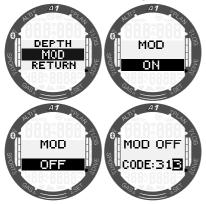
The MOD alarm uses the maximum  $ppO_2$  value which is given at the gas settings and the default value is 1.4bar.
