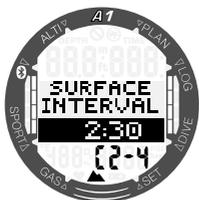
The current altitude class is shown on the left on the bottom row and the prohibited altitude is shown on the right. In the example above, the diver is presently at altitude class 2 and should not reach altitudes above 4000m (class 4) within the given interval of 2 hours and 30 minutes. By increasing the interval time on the middle row the allowed altitude increases due to the desaturation caused by the time spent at the current altitude class.
