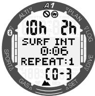
By a further press of the -/DOWN button the no-dive time (10h), no-fly time (2h), and remaining desaturation time (13:50) will be shown.
