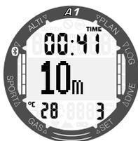
The alternative displays in APNEA mode can be scrolled by pressing the +/UP or -/DOWN buttons and this changes the dive time to the middle of the display as shown below.
