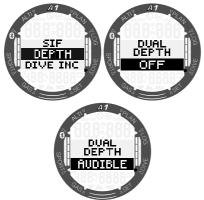
When you select depth and enable the warning by switching it to audible by first pressing the +/UP or -/DOWN buttons and then pressing the SEL/ESC button, the first depth selection is shown. By pressing the SEL/ESC button again, the second depth selection is shown.
