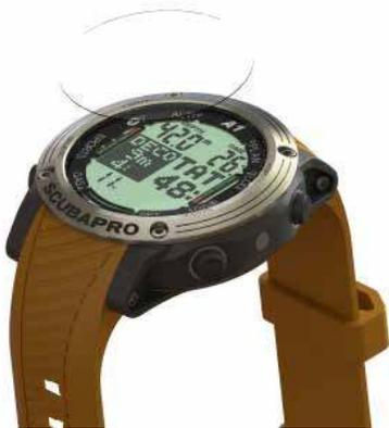
**NOTE:** If air bubbles get stuck underneath the protection foil when placing it on your A1's glass face, do not try to remove them as the water pressure will eliminate them after the first dive.
