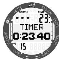
During a dive in GAUGE mode, the A1 displays depth and dive time at the top row, a timer in the middle and water temperature
