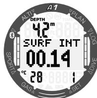
By pressing the -/DOWN button from the surface interval display, the maximum depth (4m) and duration (01.13 min) of the last dive and the total duration of the current Apnea exercise (00:04) are shown.
