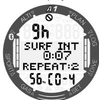
The CNS O<sub>2</sub> clock increases when the oxygen partial pressure is higher than 0.5bar, and decreases when the oxygen partial pressure is lower than 0.5bar. Hence, while on the surface breathing air you will always be decreasing the CNS O<sub>2</sub> clock. During the dive, the depth at which 0.5bar is reached for various mixes is as follows:
