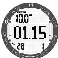
As with Gauge mode, the A1 in Apnea mode doesn't carry out any decompression calculations. You can only switch to APNEA mode if the computer is completely desaturated. Also the A1 is locked in the APNEA mode for 12 hours after shallower than 5m dives and after deeper dives the lock period is 24 hours.
