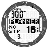
**NOTE:** The minimum depth for dive planning is 9m/30ft. The planner allows only depths in line with maximum  $ppO_2$ . The oxygen content and maximum  $ppO_2$  settings are given in the menu **GAS**.
