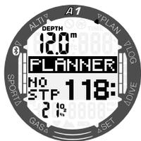
CNS% value replaces the gas mix on the bottom left of the screen when 1% would be reached for that depth with maximum no-stop time.
