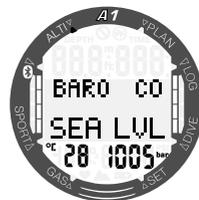
By pressing the +/UP or -/DOWN buttons you can switch to an additional display where the atmospheric pressure at sea level is shown.
