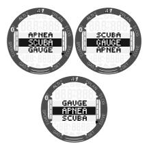
NOTE: The GAUGE and APNEA modes do not track tissue saturation so there is a locking interval before it is possible to change to SCUBA mode. In GAUGE mode the locking interval is 48h after the last dive in GAUGE mode. In APNEA mode there is a 12h locking interval with shallower than 5m/16ft dives, and a 24h locking interval with deeper than 5m/16ft dives in APNEA mode.
