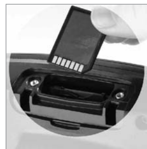
Inserting an MMC into the Card Slot
