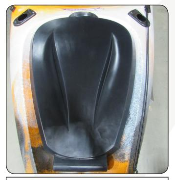
Position your Vapor 12 Kayak in a flat upright position and center the Vapor 12 Hatch(A) over the hatch opening.
