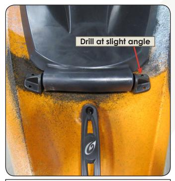
4. With the cover centered over the hatch, insert the Hatch Hinges(D) into each side of the cover. Use the hinges as a jig to drill out the rivet holes with a 13/64" Drill Bit.
