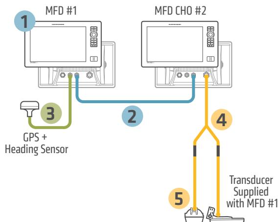
■ Ethernet ■ Transducer Cable ■ NMEA 2000
