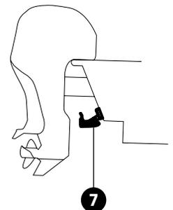
**Unobstructed View:** This jack plate installation gives the transducer safe distance from the motor and turbulence. The Side Imaging has a clear view side-to-side.
