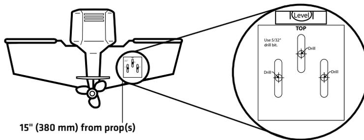
3. Continue to hold the bracket on the transom of the boat, and use a pencil or marker to mark where to drill the three mounting holes. Mark the drill holes near the top of each slot, making sure that your mark is centered in the slot.
