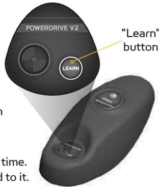
A remote can be learned to one controller at a time. A controller can have multiple remotes learned to it.
