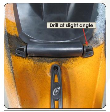
4. With the cover centered over the hatch, insert the Hatch Hinges(D) into each side of the cover. Use the hinges as a jig to drill out the rivet holes with a 13/64" Drill Bit.
