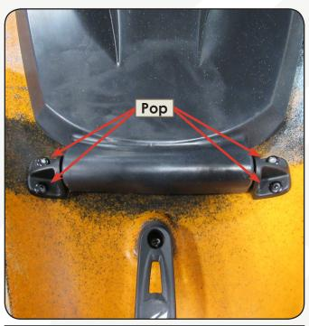
5. Insert the Cherry Rivets(B) into each hole and while pressing down on each Hatch Hinge, pop the rivets with your Rivet Gun.
