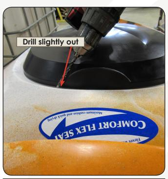
2. Using the hatch lip as a guide, drill two holes with a 1/4" drill bit into the kayak hull at a slight angle.
