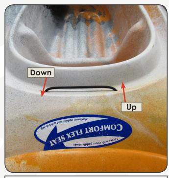
3. Knot one end of the Hatch Rope(C) and run it up through one of the newly drilled holes. Stretch it over to and down through the other hole. Tie a knot in the end of it. Both knots should be located inside the hull.
