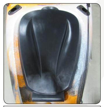
1. Position your Vapor 10 Kayak in a flat upright position and center the Vapor 10 Hatch(A) over the hatch opening.
