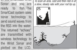
New information appears on the right. As this information moves to the left a very accurate picture of the underwater world is created, including the display of underwater objects such as the bottom, fish, and structures, as well as the depth of the bottom.
