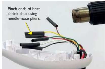
FIGURE 20 Insulate and seal six AutoPilot wires on Riptide SP motors with supplied heat shrink.
