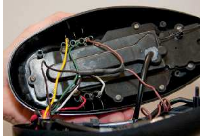
FIGURE 18 Insert AutoPilot wires into terminal holders.
