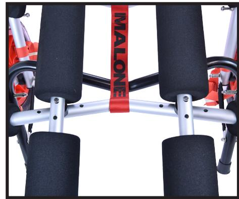
Add the straps by passing the buckle through the open loop after going around the frame as pictured. Note the strap is behind the kick-stand. See image 5
