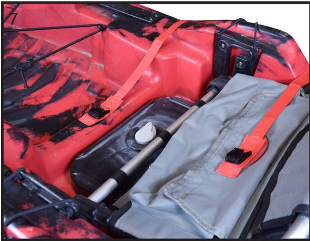
Bring the two load straps over the boat and clip together in the center. See image 7
