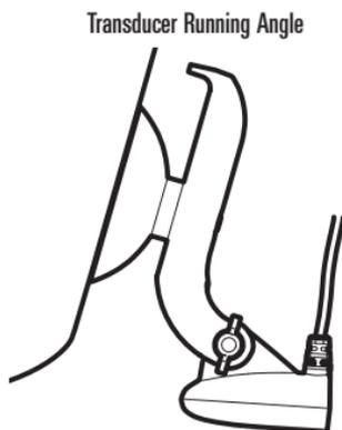
2. Adjust the running angle so that the transducer is parallel to and below the surface of the water (see the illustration *Transducer Running Angle*).
