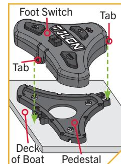
**INSTALLING THE FOOT SWITCH**
