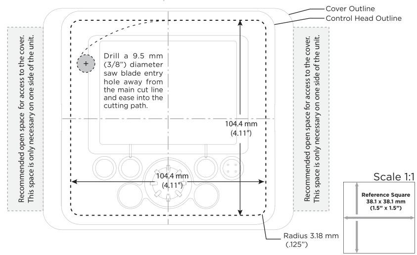
If you are reproducing or printing this template from an electronic file, set the print scale setting to None. Print the template. Measure the reference square with a ruler and adjust your reproduction setting (%) as needed so that the square measures 38.1 x 38.1 mm or 1.5" x 1.5". 531773-3 A
