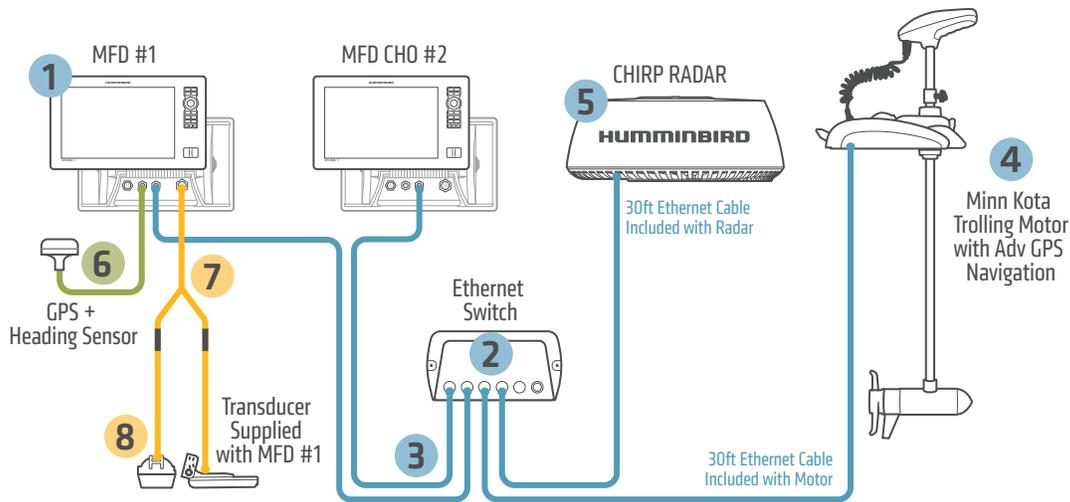
■ Ethernet ■ Transducer Cable ■ NMEA 2000
