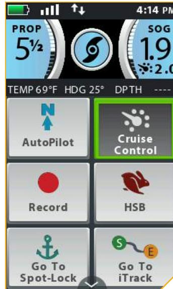
The Home Screen Buttons are Active and the Cruise Control button has been selected using the Screen Navigation
