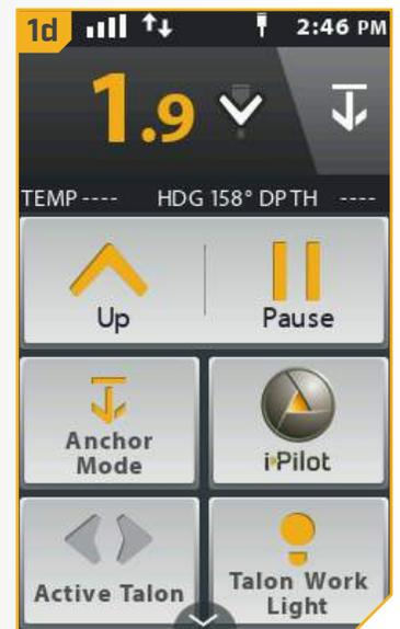
**NOTICE:** You do not need to press and hold the button to keep the Talon deploying. The Talon will automatically continue to deploy when the button is pressed until it has reached its full deployment length, received input to stop or completes anchoring.
