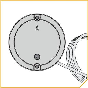
**NOTICE:** If replacement screws must be used, ensure that they are high grade non-magnetic stainless steel.
