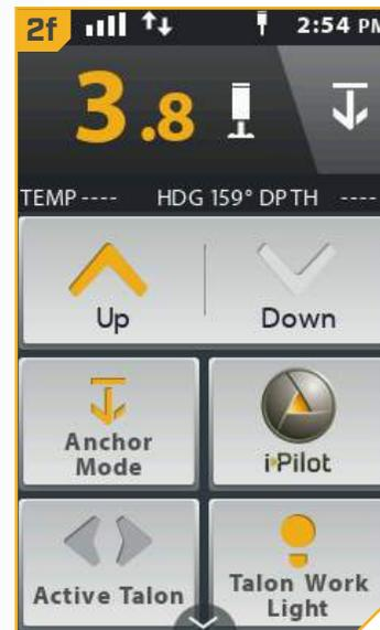
**NOTICE:** Unless the Talon Control setting on the i-Pilot Link Remote is set to Right or Left, the remote will control both Talons when deploying. Be mindful of which Talon(s) is selected when deploying them.
