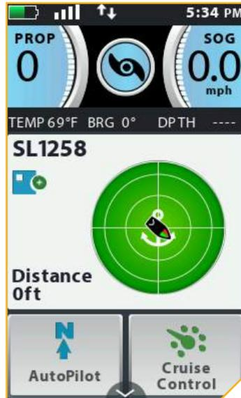
The Spot-Lock Active Band appears when Spot-Lock is engaged. The Save icon indicates that the Spot-Lock has not yet been saved.
