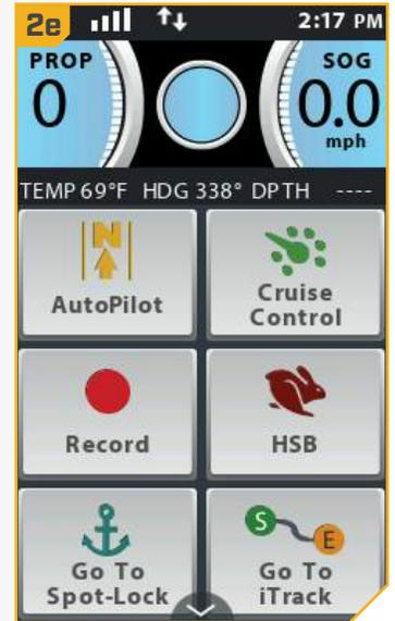
**NOTICE:** The Home Screen Buttons and appearance of the Content Area will vary slightly in appearance based on motor model and factory default selections. Home Screen Buttons can be customized. Please see "To Edit the Home Screen Button Menu" in the "Remote Controls" section of this manual.
