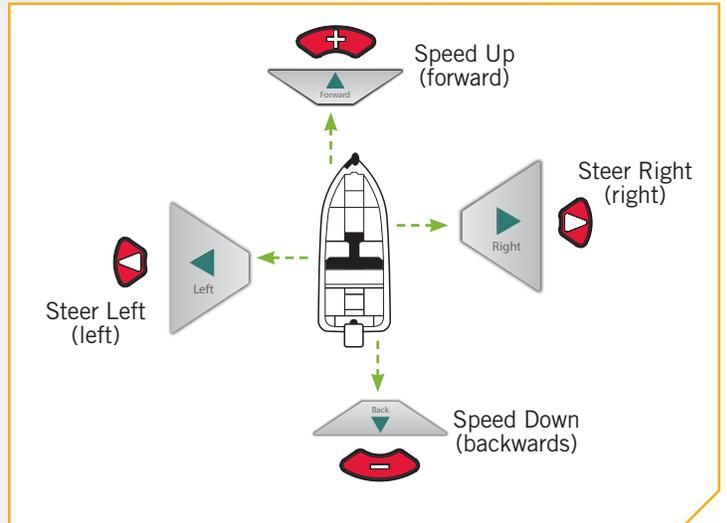
**NOTICE:** A Heading Sensor is required for Spot-Lock Jog. If your motor is not paired with a Heading Sensor, the Spot-Lock Jog directional buttons will not appear when the Spot-Lock Active Band is selected. If your motor is not paired with a Heading Sensor, the Spot-Lock location will also not Jog when the manual navigational buttons are pressed.
