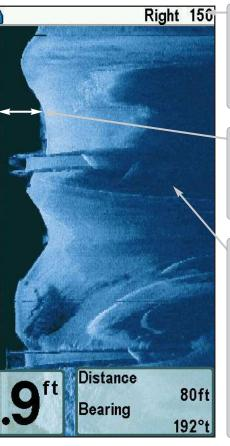
Side Imaging® Range - Images shown on the right side of the screen are located on the right side of your boat, and images shown on the left side of the screen are located on the left side of your boat. In this picture, the sonar is pinging 150 feet on each side.
