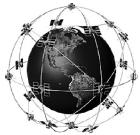
GPS uses a constellation of satellites that continually send radio signals to the earth. The GPS receiver on your boat receives signals from satellites that are visible to it. Based on time differences between each received signal, the GPS receiver determines its distance to each satellite. With distances known, the GPS receiver mathematically triangulates its own position. With once per second updates, the GPS receiver then calculates its velocity and bearing.
