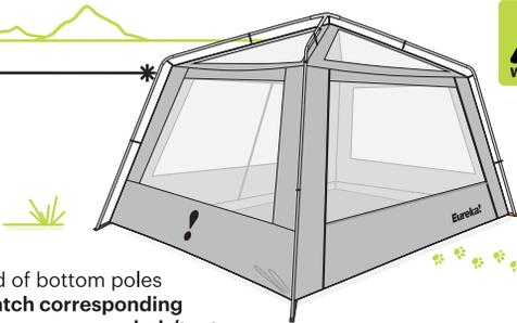
**WARNING** Ensure that peak hub, roof pole, and leg pole sticker colors match the corner webbing. Improper hub/frame alignment will damage the frame.
