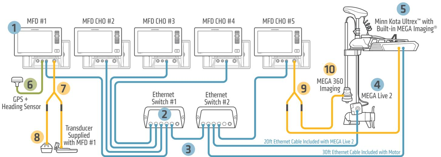
■ Ethernet ■ Transducer Cable ■ NMEA 2000
