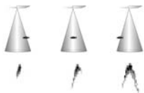
Transducer Cone and Fish Arches
