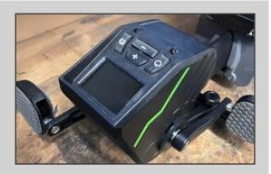
Using a 3mm hex key, remove the four screws on the face and top side of the display.
