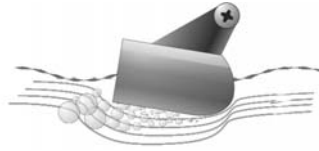
Cavitation that will cause erratic sonar readings
