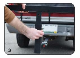
2. Insert the secondary support tube in to the primary tube. Secure with the Support Tube Hardware and Lock Pin.
