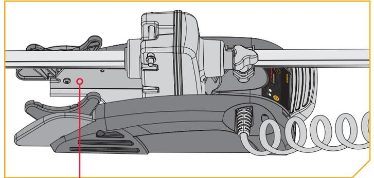
**NOTICE:** The serial number on your Kayak Terrova is located inside the mount below the motor rests.
