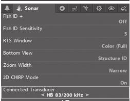
Use the following instructions to set up an accessory transducer the first time the control head is powered on. Once the transducer is set up in the system, you will only have to repeat these instructions if you restore the control head defaults or update the software.
