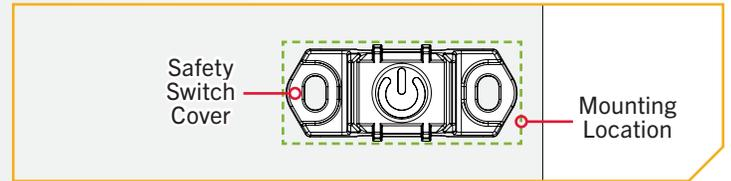
**NOTICE:** Select watercraft models may have a molded standoff for the Safety Switch Wire and Cover. If a molded standoff is present, placing the masking tape, drilling a hole for the Wire, and installing the Spacer (Item #10) may be unnecessary.
