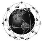
GPS uses a constellation of satellites that continually send radio signals to the earth. The GPS receiver on your boat receives signals from satellites that are visible to it. Based on time differences between each received signal, the GPS receiver determines its distance to each satellite. With distances known, the GPS receiver mathematically triangulates its own position. With 5 updates per second, the GPS receiver then calculates its velocity and bearing.
