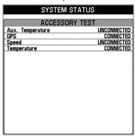
**NOTE:** The speed accessory will be detected only if the paddlewheel has moved since your Fishfinder was powered up.
