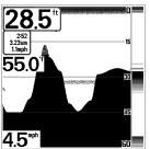
**Black** (Bottom Black) displays all pixels below the bottom contour as black, regardless of signal strength. This has the benefit of providing a high contrast between the bottom and other sonar returns on the display.
