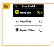
**NOTICE:** The radio button next to the desired function will be selected when the Steer Right button is used to customize the function. AutoPilot is the default selection for Ulterra QUEST and Riptide Instinct QUEST series trolling motors. The function options listed are based on the trolling motor and other devices in the Advanced GPS Navigation network.
