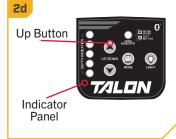
**NOTICE:** Once the Talon is put into Manual Retract Mode, it will stay in this mode for 30 minutes.
