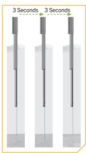
NOTICE: Attempting to retract the Talon before it has completed its automated deployment sequence, will only cancel the deployment sequence in process, and not retract the Talon. You may retract the Talon normally when a deployment sequence has been completed or canceled.
