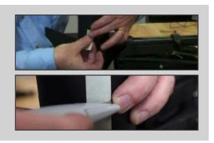
Use the 1/4" nut driver to remove the two 1/4" thru bolts. Remove the motor end housing by pulling it up and off the motor shaft.
