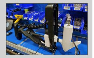
Visually inspect the area behind the prop hub for any evidence of fishing line or debris wrapped around the prop shaft or damage to the prop shaft seals.
