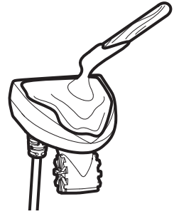
Applying Epoxy to the 200/83 kHz Transducer
