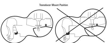
**Unobstructed View:** The jack plate gives the transducer safe distance from the motor and turbulence. The Side Imaging™ has a clear view side-to-side.
