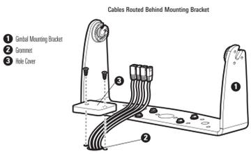
10. Thread the cables through the opening in the back of the cable collector cover.
