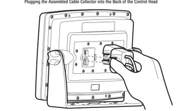
5. **Gimbal Mount:** Place the control head back onto the mounting bracket. Adjust the control head to the desired viewing angle and secure by tightening the gimbal knobs.
