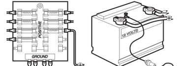
The control head power cable can be connected to the electrical system of the boat at one of two places: a fuse panel usually located near the console, or directly to the battery.
