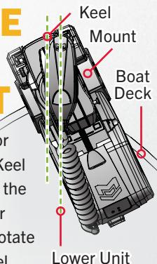
The trolling motor comes with the Keel Offset parallel to the motor mount. For proper control, rotate the motor parallel to the boat's Keel and set the Keel Offset. Record the Keel Offset through the One-Boat Network app or Wireless Remote.
