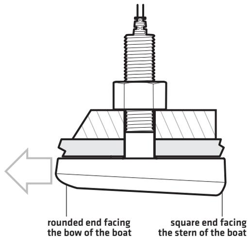
2. Insert the transducer into the drilled hole from outside the boat with the leveling block[s] installed according to your installation type.
