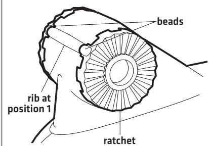
**Ratchets Placed in Position 2**
