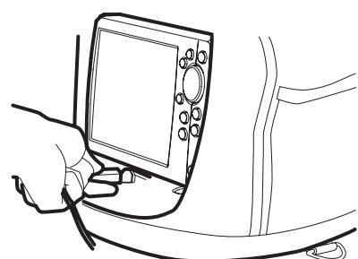
the Sonar/Speed Y-Cable connector into the jumper port in the portable case. Then, connect the transducer connector and speed sensor connector to the corresponding connectors on the Y-Cable. The Y-Cable requires a separate purchase. Contact Humminbird Technical Support for details.
