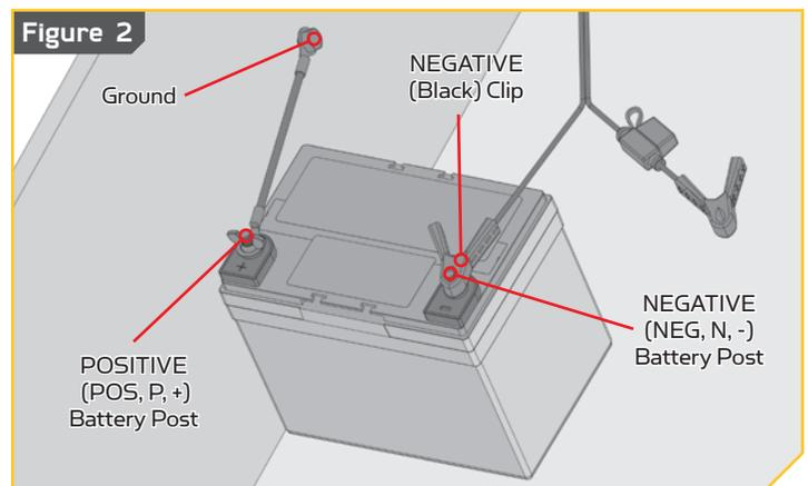
16. FOLLOW THESE STEPS WHEN BATTERY IS OUTSIDE VEHICLE. A SPARK NEAR THE BATTERY MAY CAUSE BATTERY EXPLOSION. TO REDUCE RISK OF A SPARK NEAR BATTERY:
