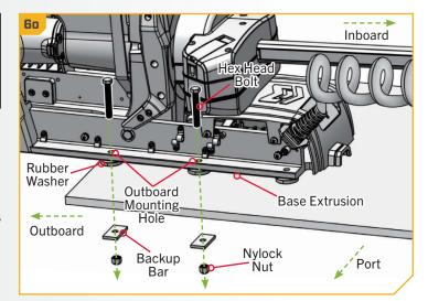
**NOTICE:** Use extra care to avoid pinching and damaging the sensor wires that run alongside the Base Extrusion when installing and tightening the mounting hardware.
