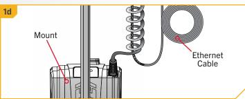
**NOTICE:** Minn Kota recommends routing the Ethernet Cable through the Coil Cord. Bypassing the Coil Cord when routing the Ethernet Cable is not recommended.
