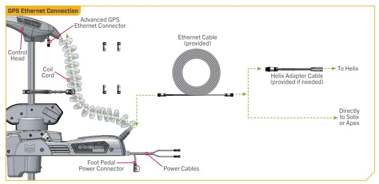
**NOTICE:** Minn Kota recommends routing the Ethernet Cable or Ethernet Extension Cable through the Coil Cord when making the Ethernet connection. The cable will be installed from the Mount to the Control Head through the Coil Cord. Bypassing the Coil Cord when routing the Ethernet Cable or Ethernet Extension Cable is not recommended.
