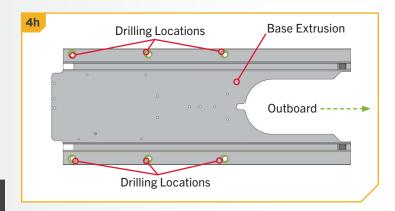
**NOTICE:** The mounting surface for the Riptide Instinct QUEST must be flat. Rubber Washers can be used to shim the Base Extrusion flat before hardware is tightened.
