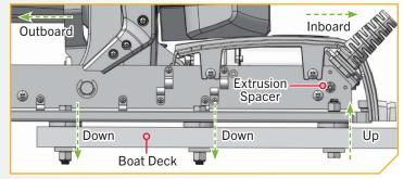
Replace the Right Sideplate and Left Sideplate. Replace the four Sideplate Screws using a #3 Phillips Screwdriver. Two of these screws will be located on each side of the mount.
