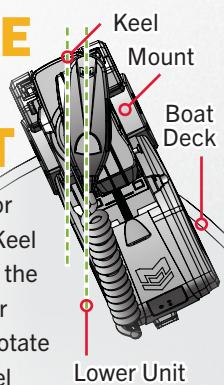
The trolling motor comes with the Keel Offset parallel to the motor mount. For proper control, rotate the motor parallel to the boat's Keel and set the Keel Offset. Record the Keel Offset through the One-Boat Network app or Wireless Remote.
