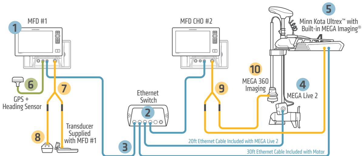
■ Ethernet ■ Transducer Cable ■ NMEA 2000
