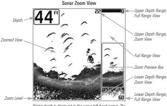
Digital depth is displayed in the upper left hand corner. The digital readouts in the Sonar Zoom View cannot be customized; therefore, information such as water temperature and voltage are unavailable in the Sonar Zoom View.
