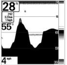
**Black** (Bottom Black) displays all pixels below the bottom contour as black, regardless of signal strength. This has the benefit of providing a high contrast between the bottom and other sonar returns on the display.
