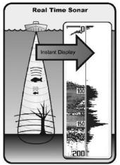
SONAR is an acronym for SOund and NAvigation Ranging. Sonar utilizes precision sound pulses or "pings" which are emitted into the water in a teardrop-shaped beam.
