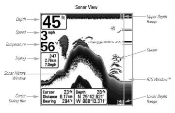
**NOTE:** If the Depth number is flashing, it means that the unit is having trouble locating the bottom. This usually happens if the water is too deep, the transducer is out of the water, the boat is moving too fast, or for any other reason that the unit can't accurately receive continuous data.
