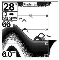
**NOTE:** Selecting Simulator from the Start-Up Options Menu allows you to pre-configure your Fishing System for on the water operation. Any menu changes you make will be saved for later use.
