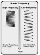
The sound pulses are transmitted at various frequencies depending on the application. Very high frequencies (455 kHz) are used for greatest definition but the operating depth is limited. High frequencies (200 kHz) are commonly used on consumer sonar and provide a good balance between depth performance and resolution. Low frequencies (83 kHz) are typically used to achieve greater depth capability.
