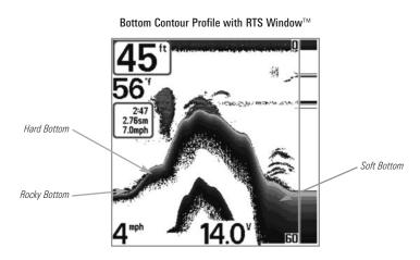
The sonar returns from the bottom, structure, and fish can be represented as either **Inverse**, **Structure ID®**, **WhiteLine™**, or **Black** (Bottom Black). See **Sonar X-Press™ Menu: Bottom View** for details on how to set the bottom view.
