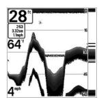
**Inverse** is a method where weak returns are shown with dark pixels and strong returns with lighter pixels. This has the benefit of ensuring that weak signals will be clearly visible on the display.
