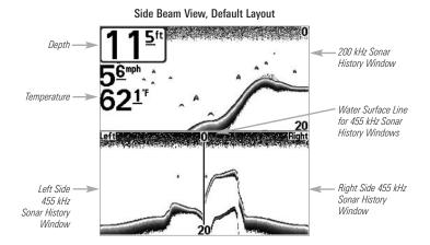
**Classic layout:** The top portion of the display presents a historical log of sonar returns from the 200 kHz down-looking sonar beam. New information in the down beam panel scrolls from right to left. The bottom portion of the display presents a historical log of sonar returns from the 455 kHz right- and left-looking sonar beams. New information appears at the top, and scrolls down the display.
