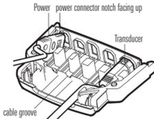
**CAUTION!** It is important to place the connectors into the correct slots and right side up. See the illustration **Locating the Cable Tray Slots** for details.
