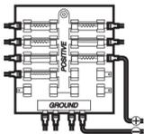
**Battery Connection:** Install an inline fuse holder (not included) and the required fuse (as shown in the **Required Fuse Size** table). Attach the black wire to ground (–), and the red wire to positive (+) 12 VDC power.
