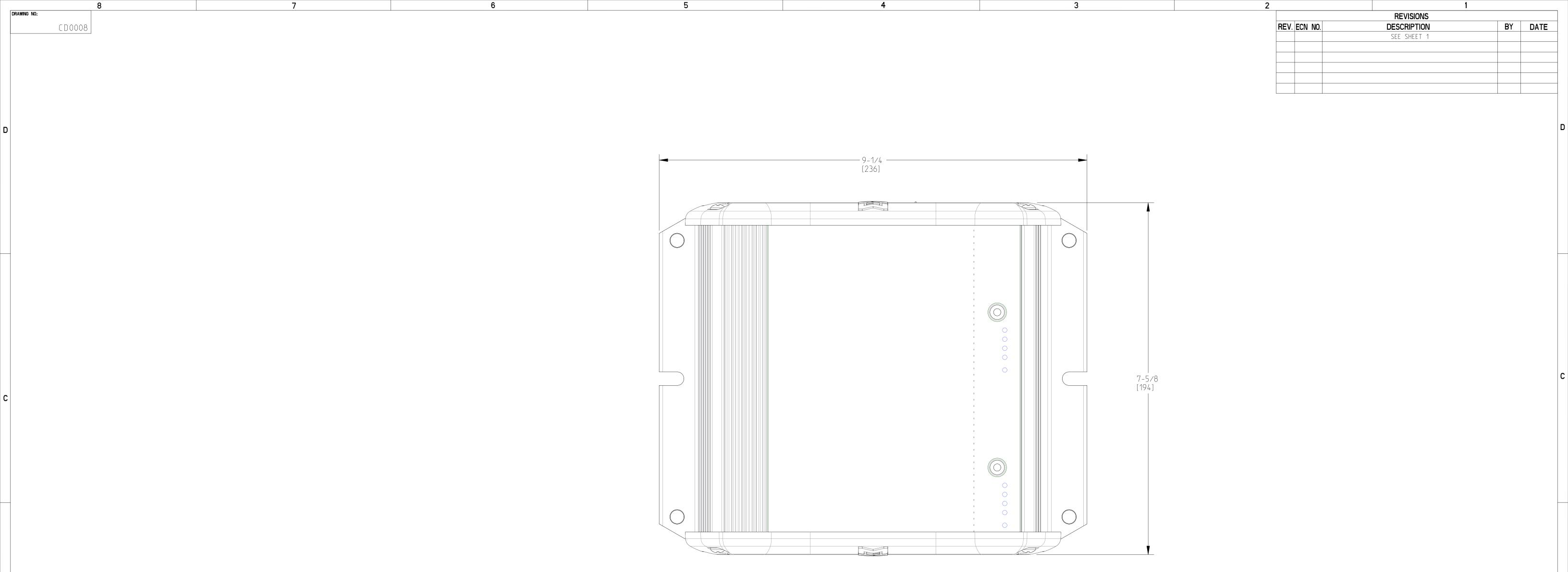
MAINTAIN SIX INCHES OF CLEARANCE ON ALL SIDES OF CHARGER FOR PROPER AIR CIRULATION AND COOLING
