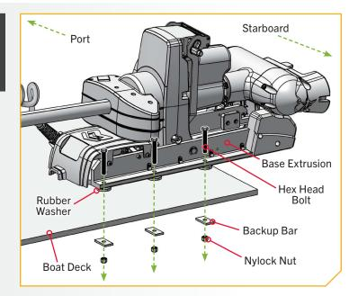
**NOTICE:** Use extra care to avoid pinching and damaging the sensor wires that run alongside the Base Extrusion when installing and tightening the mounting hardware.
