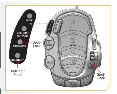
**NOTICE:** If the Spot-Lock button is accidentally pressed, press the Spot-Lock button again to cancel Spot-Lock.
