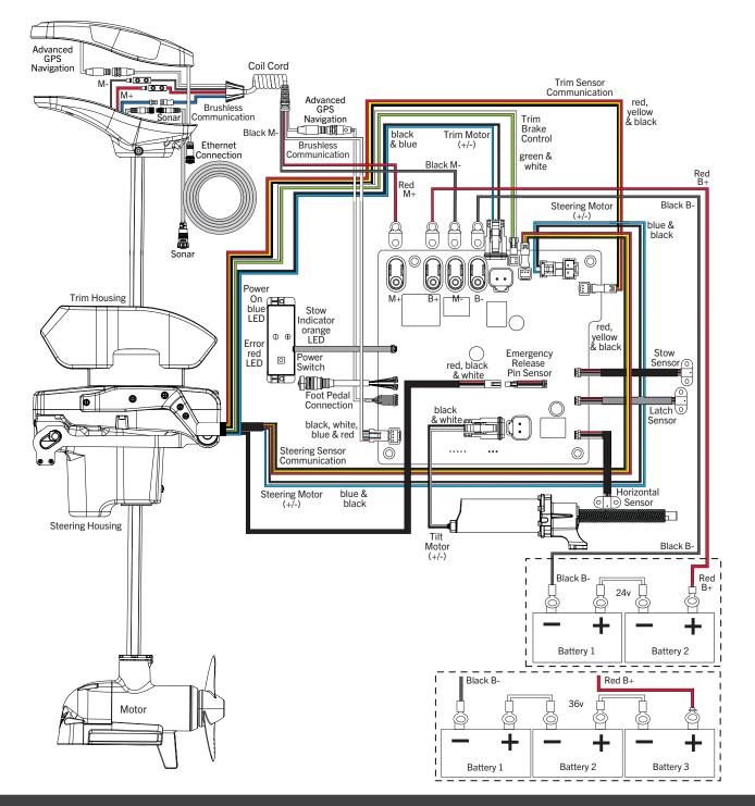
**NOTICE:** This is a multi-voltage diagram. Double-check your motor's voltage for proper connections. Over-Current Protection Devices are not shown in this illustration.
