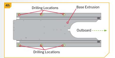
**NOTICE:** The mounting surface for the Ulterra QUEST must be flat. Rubber Washers can be used to shim the Base Extrusion flat before hardware is tightened.
