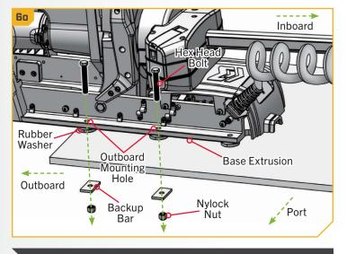
**NOTICE:** Use extra care to avoid pinching and damaging the sensor wires that run alongside the Base Extrusion when installing and tightening the mounting hardware.
