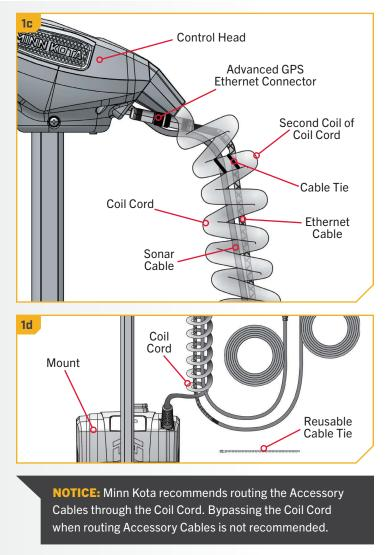
**NOTICE:** The Ethernet Cable should be secured to the second coil of the Coil Cord. Securing the Ethernet Cable to any other coil may damage the Cables.
