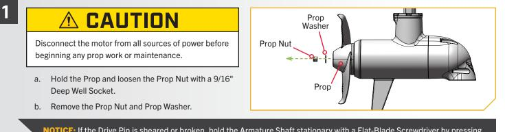
**NOTICE:** If the Drive Pin is sheared or broken, hold the Armature Shaft stationary with a Flat-Blade Screwdriver by pressing into the slot on the end of the shaft while loosening the Prop Nut.
