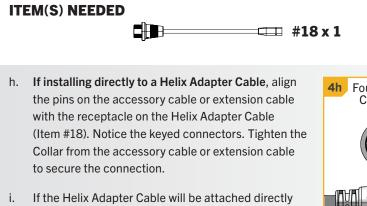
to a Humminbird<sup>®</sup> Helix, plug it in the Helix Adapter Cable Keyed Connection on the back of the fish finder.
