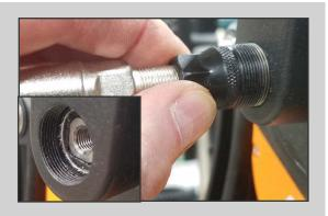
Note how the worn threads in the previous photo are no longer visible on this properly set puller.
