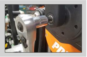
Note the threads on the perimeter of the opening in the crank arm. Turn the black, threaded end of the crank arm puller tool (C) into these threads until bottomed out.
